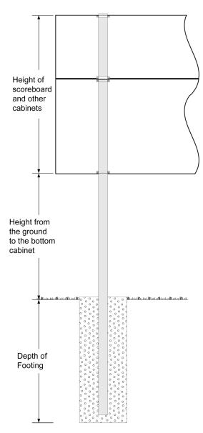
The length of your posts is determined by the configuration of your scoreboard display, its height above the ground, and the depth of your footings. Footing size is also related to the cabinet height and configuration. To some degree, the depth of the footings will be determined by the equipment available to the installer. In general, a smaller diameter hole needs to go deeper than a larger diameter hole. The trick is to create footings hefty enough to provide stability for the sign structure.
